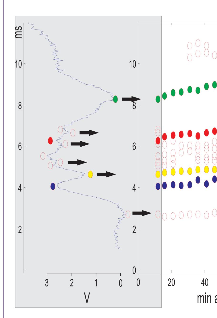
**7.** The signal propagation tends to slow down during the course of the anaesthesia.
