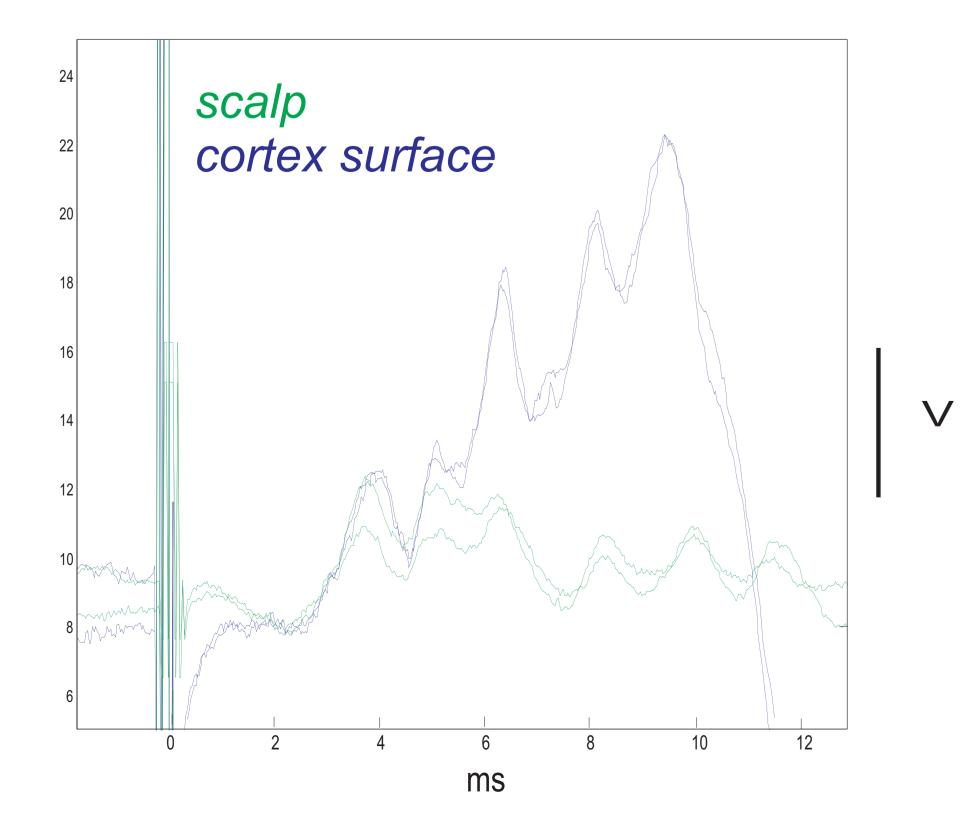
SEPs obtained with electrodes placed either on the scalp or in contact with the dura in one animal during two different sessions.
