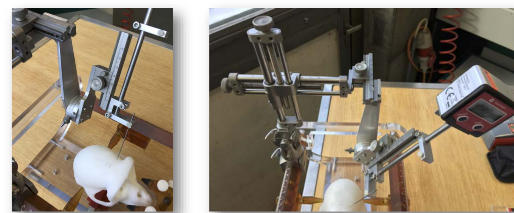
Pictures of the micro-manipulator with different additional pieces (Rotator adaptor and vernier). University of Fribourg (2017)
