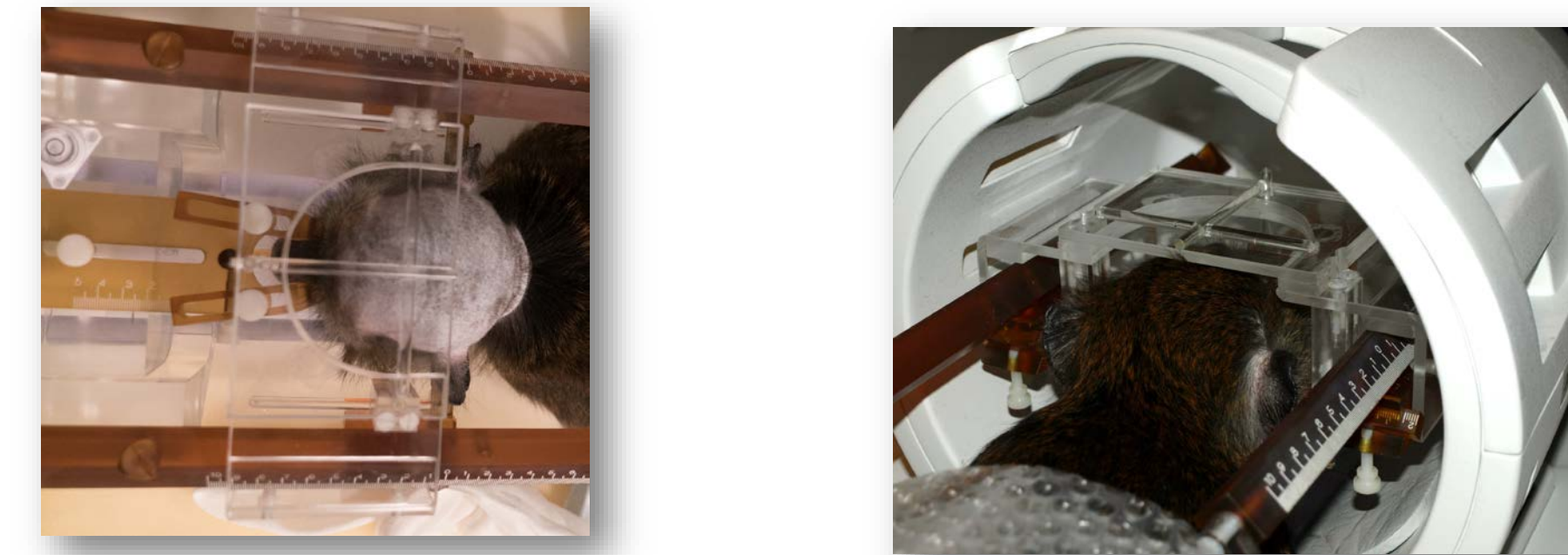
Developed MRI-localizer attached to a standard stereotaxic frame. University of Fribourg (2016)
