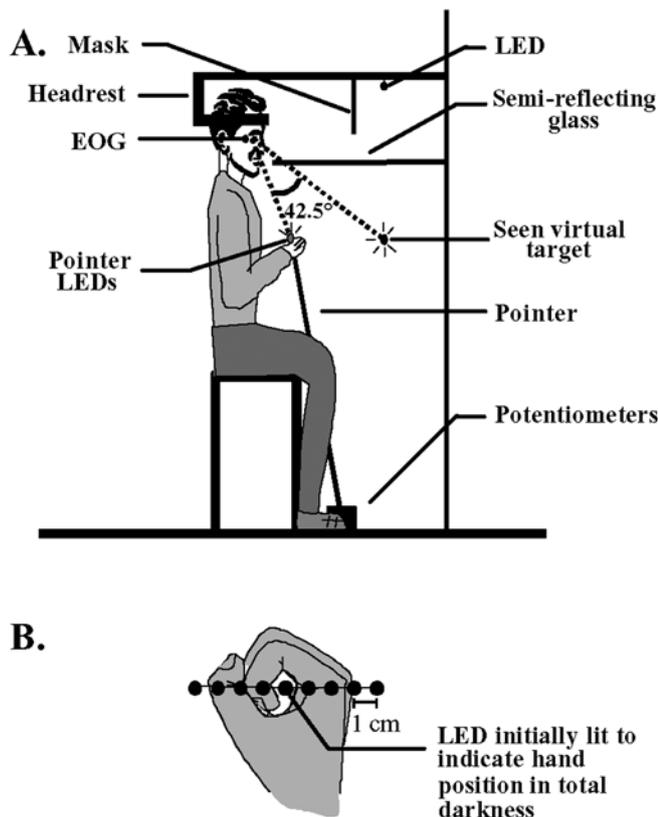
**Fig. 1** A Side view of the apparatus. B Top view of the nine LEDs that were used to provide true or erroneous visual feedback on hand position in complete darkness. Only one LED was lit at the same time
