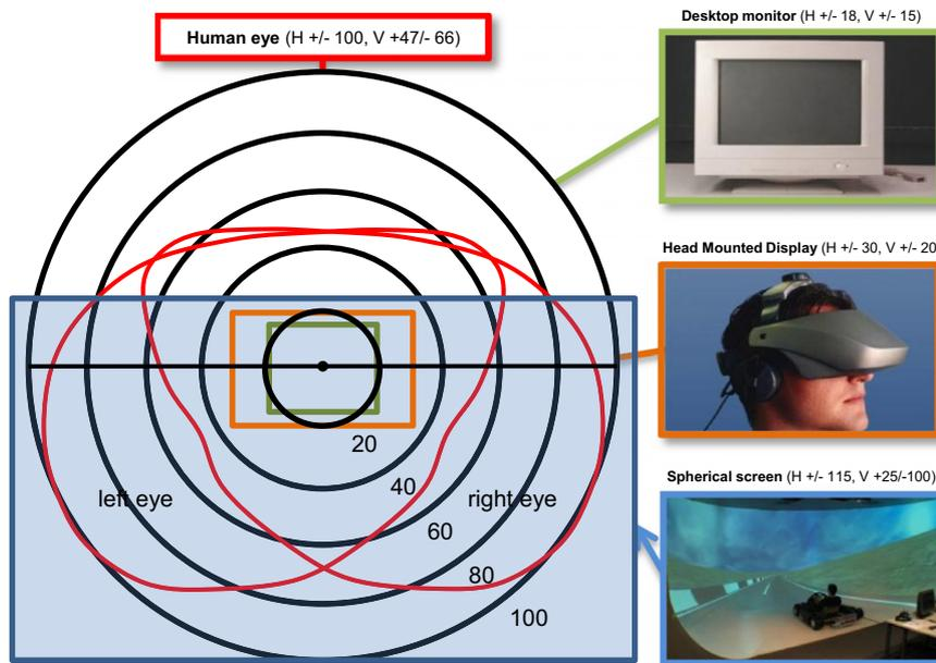
**Fig. 1.** Field of view in degrees of different setups compared to the human field of view (drawn after a graphic from CHI Data Visualization '<http://www-users.cs.umn.edu/~echi/tutorial/perception2000/>').
