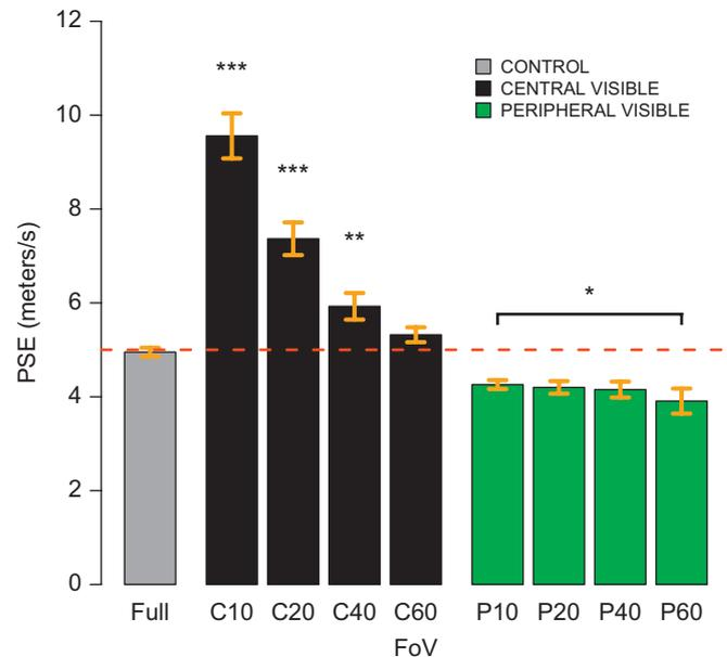
**Fig. 11.** PSE mean values as a function of the FoV. The red dashed line corresponds to the actual speed of the standard stimulus.
