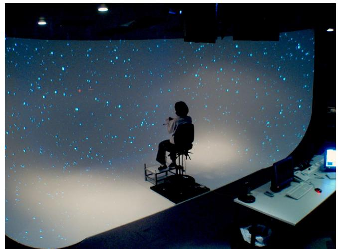
**Fig. 2.** Panoramic screen, 230 × 125° of field of view, including floor.
