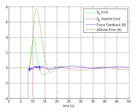
Fig. 7 - DHA without Pilot in the loop Simulation. Altitude response (brown line). The DHA Simulator by itself is piloting the aircraft. The green line shows the operator input. The blue line shows the net sum of haptic aiding and spring force.
