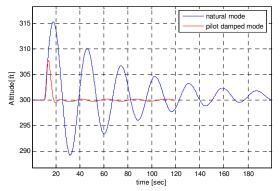
Fig. 1 - Phugoid natural aircraft mode (blue line) versus the typical aircraft response damped by a good pilot (red line).
