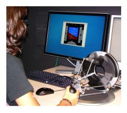
Fig. 9 - Picture of the test setup, showing the display and the haptic device.
